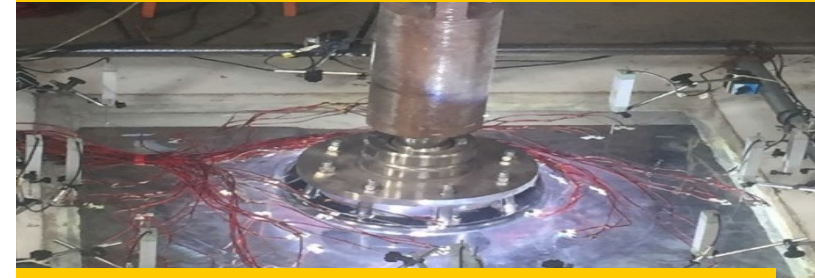
Load test of node: break at 100 tons
