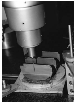
FIGURE 4. Geometric measuring on a large three-plate neutron interferometer.
