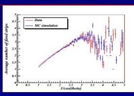
Fig. 6. Hit strip multiplicity vs  $\,1/cos\theta$  and MC comparison
