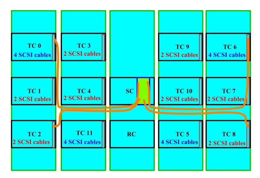
Cables length(max) => 1m + 2\*.5m + .5m = 2.5m total number of SCSI cables => 32 cables
