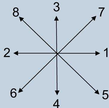
$f_i(\vec{x}, t)$  = particle density at site  $x$  at time  $t$  with  $i$ -th velocity
