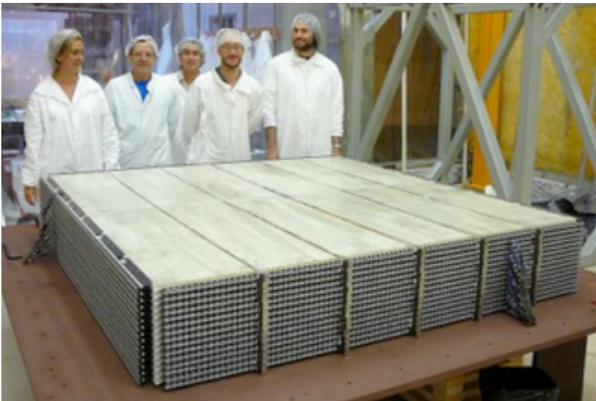
Stacked scintillator XY modules for FGD1
