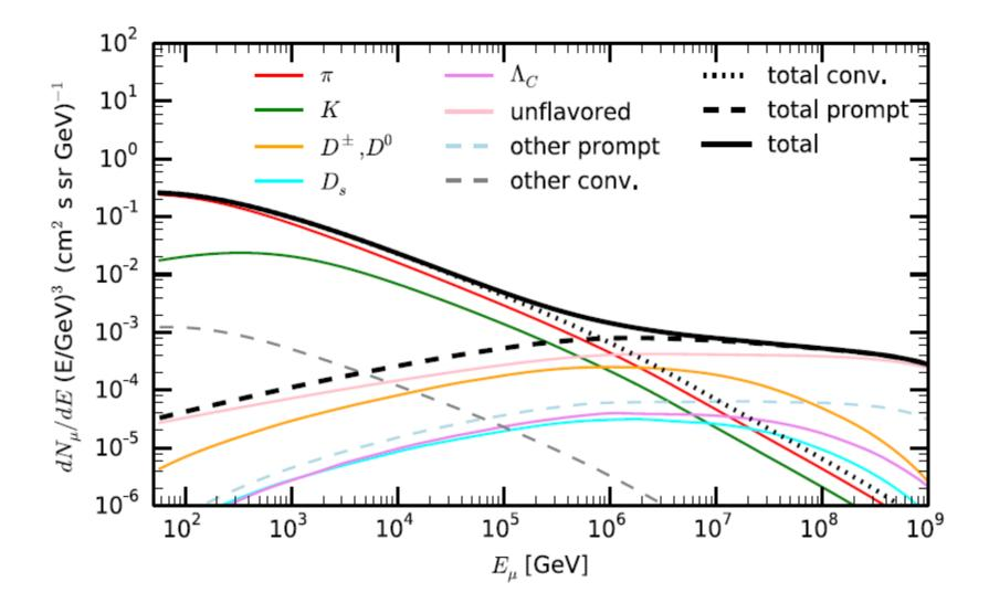
Contribution of different particle decays to the atmospheric muon flux. Note that the prompt muons start dominating over the conventional muon fluxes above 1 PeV, Note that the muon fluxes are multiplied by the muon energy cubed.
