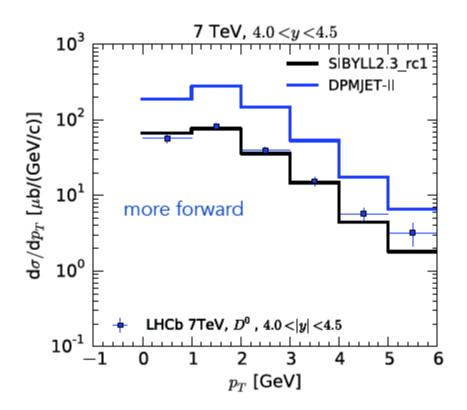
We compared our predictions for charm production at LHC to those of DPMJET II. While in the central region the two predictions are similar, in the central and forward regions DPMJET generates many more charm particles, while Sibyll is consistent with the experimental data in the whole phase space.
