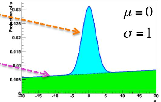
$$\tilde{f}_{sig}(x) = \frac{1}{\sqrt{2\pi\sigma^2}} e^{-\frac{1}{2}\left(\frac{x-\mu}{\sigma}\right)^2} \quad (\text{banalmente si elimina il coeff. multiplicative A})$$
